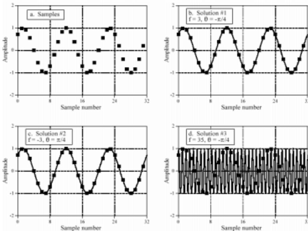
FIGURE 10-11 The meaning of negative frequencies. The problem is to find the frequency spectrum of the discrete signal shown in (a). That is, we want to find the frequency and phase of the sinusoid that passed through all of the samples. Figure (b) is a solution using a *positive* frequency, while (c) is a solution using a *negative* frequency. Figure (d) represents a family of solutions to the problem.
