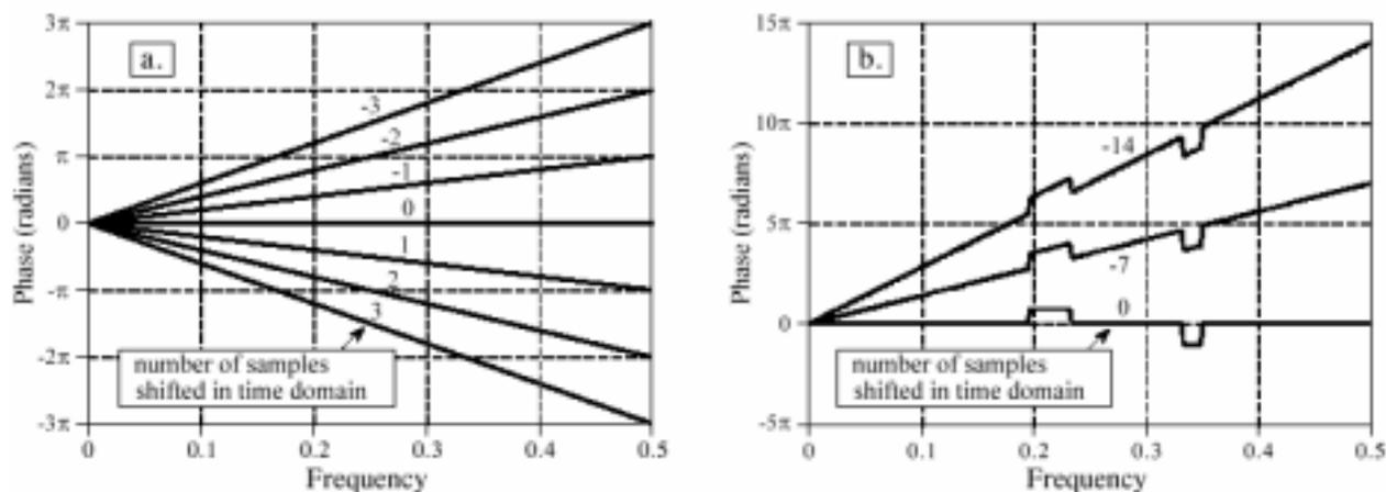
FIGURE 10-5. Phases resulting from time domain shifting.
