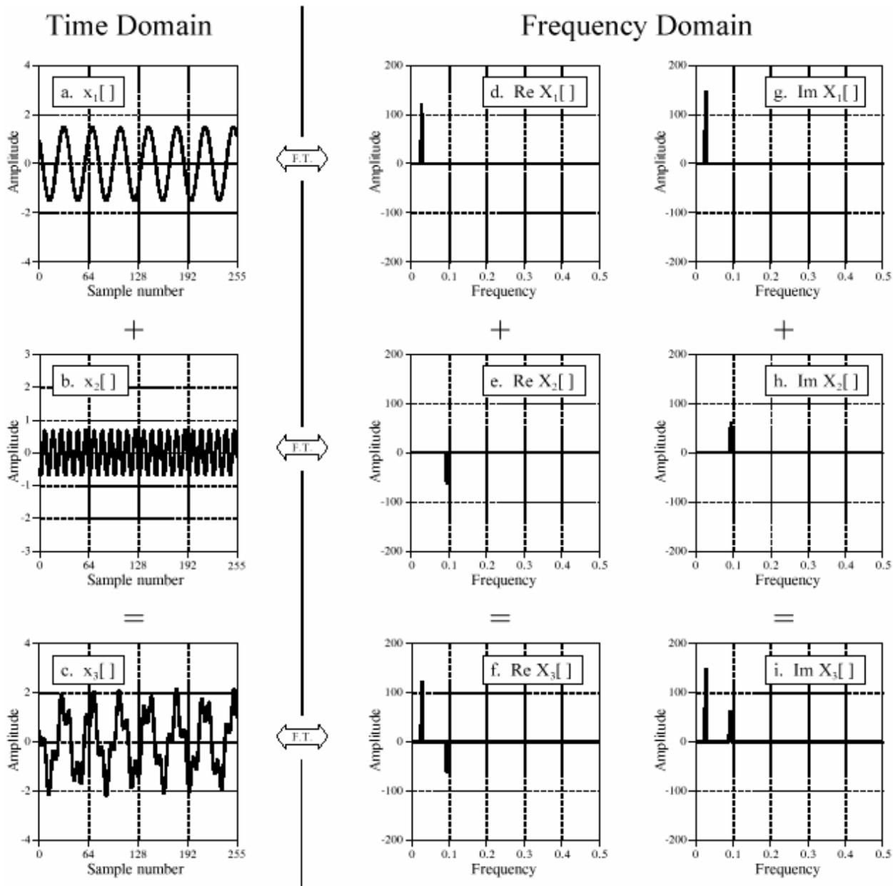
Figure 10-2. Additivity of the Fourier transform. Adding two or more signals in one domain results in the corresponding signals being added in the other domain. In this illustration, the time domain signals in (a) and (b) are added to produce the signal in (c). This results in the corresponding real and imaginary parts of the frequency spectra being added.
