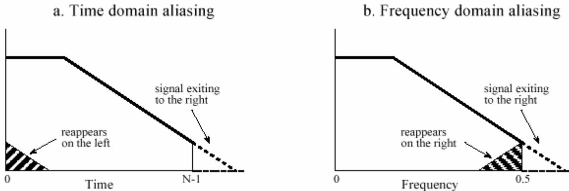
FIGURE 10-10 Examples of aliasing in the time and frequency domains, when only a single period is considered. In the time domain, shown in (a), portions of the signal that exit to the right, reappear on the left. In the frequency domain, (b), portions of the signal that exit to the right, reappear on the right as if they had been folded over.
