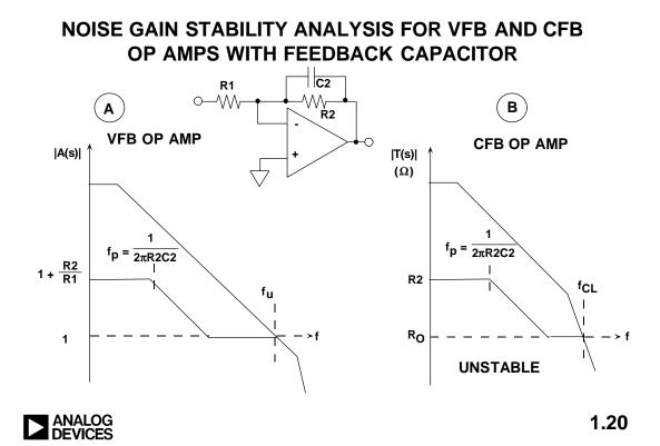
In the case of the CFB op amp (Figure 1.20b), the same analysis is used, except that the open-loop transimpedance gain, T(s), is used to construct the Bode plot. The definition of *noise gain* (for the purposes of stability analysis) for a CFB op amp, however, must be redefined in terms of a *current* noise source attached to the inverting input (see Figure 1.21). This current is reflected to the output by an impedance which we define to be the "current noise gain" of a CFB op amp:
