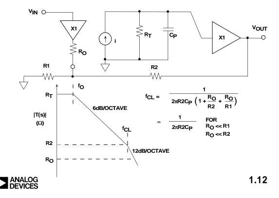
The finite output impedance of the input buffer is modeled by Ro. The input error current is *i*. By applying the principles of negative feedback, we can derive the expression for the op amp transfer function:
