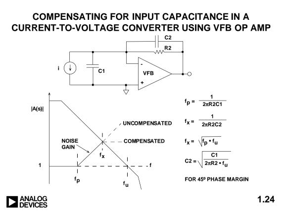
The net input capacitance, C1, forms a pole at a frequency  ${\rm f}_p$  in the noise gain transfer function as shown in the Bode plot, and is given by:
