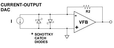
\* NOT REQUIRED FOR CFB OP AMP BECAUSE OF LOW INVERTING INPUT IMPEDANCE
