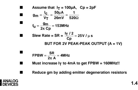
In practice, the FPBW of the op amp should be approximately 5 to 10 times the maximum output frequency in order to achieve acceptable distortion performance (typically 55-80dBc @ 5 to 20MHz, but actual system requirements vary widely).
