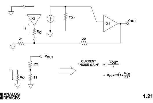
Now, return to Figure 1.20b, and observe the CFB *current noise gain* plot. At low frequencies, the CFB current noise gain is simply R2 (making the assumption that Ro is much less than Z1 or Z2. The first pole is determined by R2 and C2. As the frequency continues to increase, C2 becomes a short circuit, and all the invertig input current flows through Ro (refer back to Figure 1.21).
