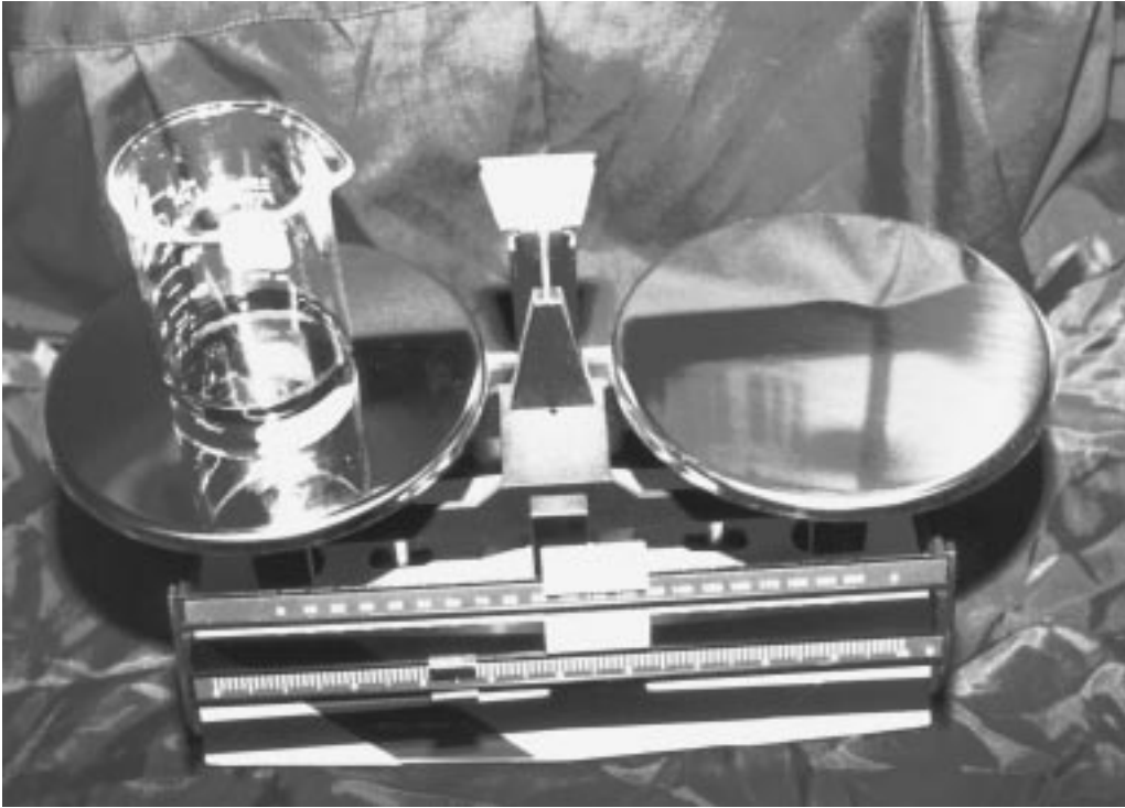
FIGURE 20.2 Beam balance. (Courtesy Denver Instrument Company.)
